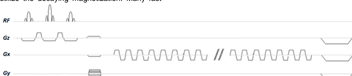
Fig. 1: The sequence diagram of 2D SSSP-EPSI with three sub-pulses in the excitation and echo planar readout in one of the two spatial directions.
